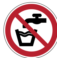
Eau non potable P005
